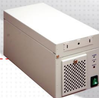
Industrial PC with AVT's video capture card
